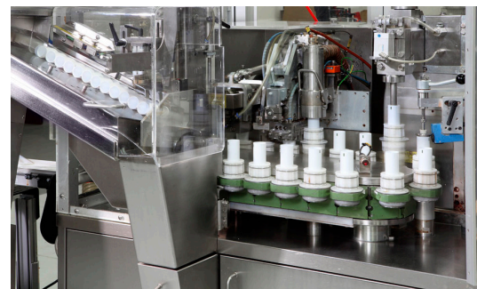
Tri-Pac Line 8 – Tube Filling Line
